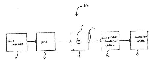
(57) Abstract: Disclosed are methods of cleaning articles of manufacture using hydrofluorocarbon and hydrochlorofluorocarbon fluids. The methods comprise generally the steps of (a) providing a hydrofluorocarbon and/or hydrochlorofluorocarbon fluid in liquid or supercritical state; (b) contacting an article of manufacture with said fluid; and (c) removing substantially all of said fluid from said article of manufacture.
