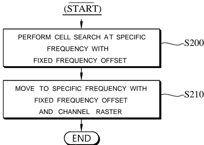
(57) **Abstract:** A method and apparatus for performing a cell search in a wireless communication system is provided. A narrowband user equipment (NB UE) performs the cell search at a specific frequency with a fixed frequency offset, and moves to the specific frequency with the fixed frequency offset and a channel raster.
