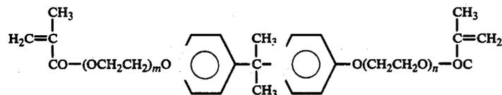
This liquid monomer, 2,2-bis[(4-methacryloxy polyethoxy)phenyl]propane, (hereinafter referred to as "Bis-MPEPP") is then mixed with powders of methacrylic resin polymers to form a slurried product which is found to have a substantially improved workability and provide excellent physical properties to the end product and, therefore, to be well suited for the resinous materials for restoring crowns.
