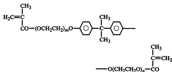
wherein the average molar amount of ethylene oxide units (m + n), present satisfies the relation: 2.2 ≤ (m + n) ≤ 6, and a powder component B which is a methacrylic resin polymer, wherein said liquid component A is mixed with said powder component B in proportions ranging from 1:3 to 4:1.
