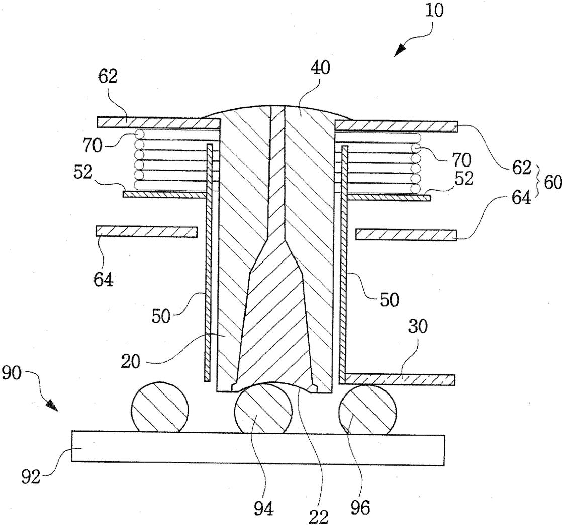
**TEST PROBE FOR SEMICONDUCTOR PACKAGE**
